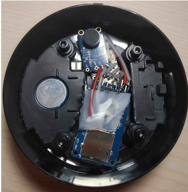
Figure 7.11: Spy Bug placed inside the Echo Dot.
