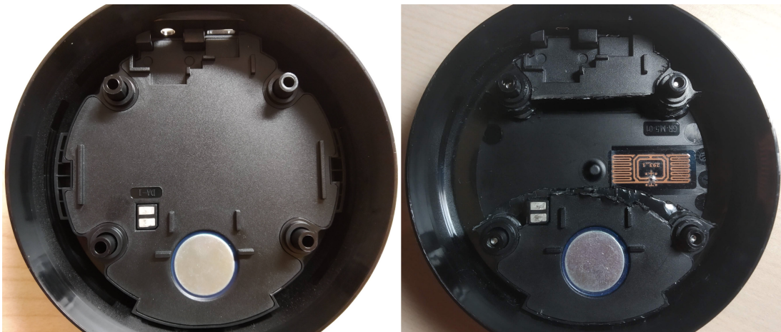
Figure 7.9: Echo Dot's "acoustic chamber" before and after I removed some of the plastic casing. The bits of it that I left in keep the speaker and the ports in place.
